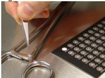
6. Using the round end of the purple applicator tool, apply firm pressure to the center of the KeyDot and work towards the outside in a circular motion. This pressure activates the pressure-sensitive adhesive and smooths the edge of the KeyDot. Alternatively, you can apply firm pressure to the KeyDot using an index finger, while wearing gloves, to activate the adhesive.
