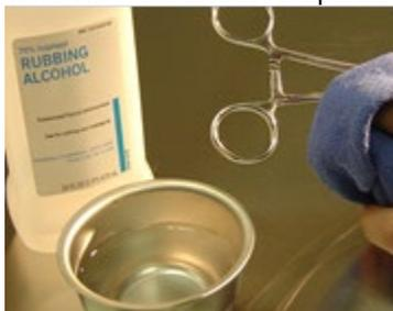
5. Once the alcohol has dried, use tweezers or forceps to remove the KeyDot from the KeyDot sheet and immediately apply it to the selected location. Do not touch the exposed adhesive of the KeyDot or the cleaned area of the instrument. Unclean surfaces, from oils and debris on fingers, can interfere with successful bonding.
